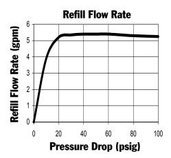
**NOTE:** The 454 3/4" Control Flow Brine Valve is designed for salt brine only. It will also fit inside a brine well that is 5" or larger.
