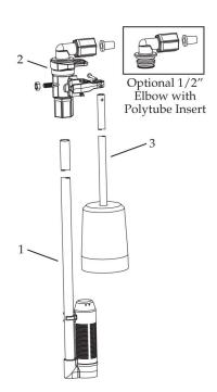
The 474 Safety Brine Valve System consists of three components which must be ordered separately:
