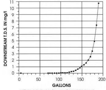
(Calculated using Reverse Osmosis Water at 32 mg/l and a flow rate of 0.1 gpm).
